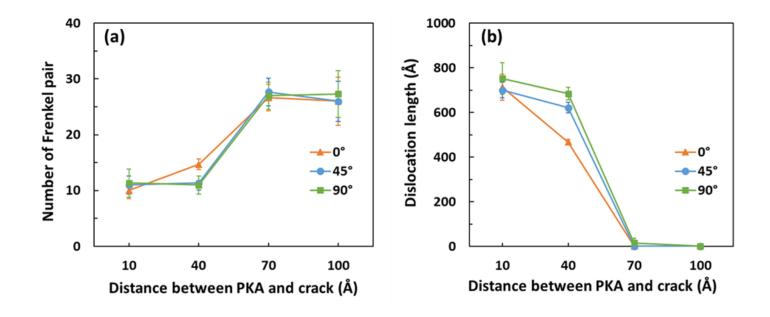
the number of Frenkel pairs is significantly increased when the PKA distance is increased from 40 Å to 70 Å.
