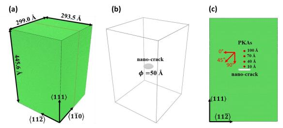
Configuration of simulation cell-Ni single crystal with a nanoscale crack
