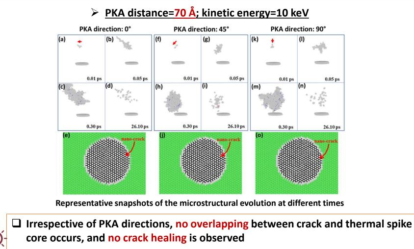
After equilibration, the radiation damage is mainly in the form of point defects, almost no dislocation loop and stacking fault can be observed
